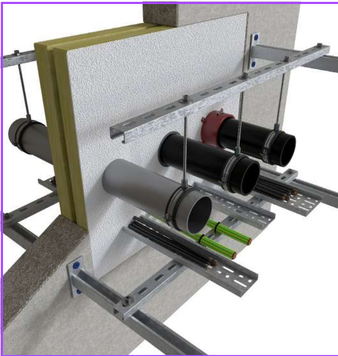
Figure 21 Multiple services within a single opening
