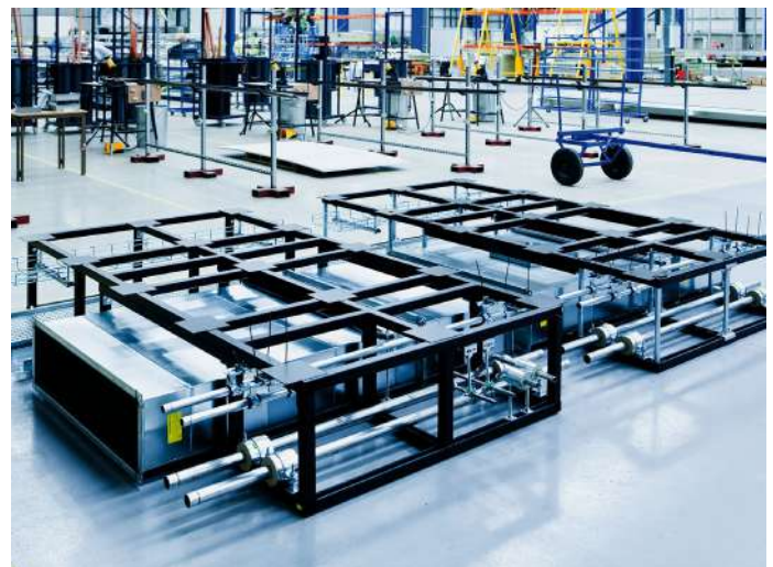
Figure 4 Example of a prefabricated corridor M&E module
